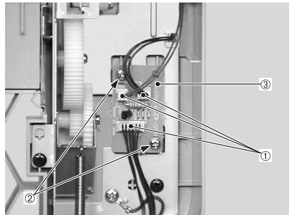
① Connectors ② Screws ③ Paper feeder PCB
